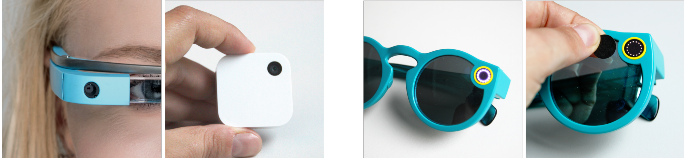
Figure 1. For bystanders it is not always easy to determine whether state-of-the-art body-worn cameras are recording them: some devices, such as Google Glass (left) or the Narrative Clip (2nd from the left) do not provide any status indicator or privacy notice. Other devices, e.g., the Snap's Spectacles (2nd from the right), provide LED indicators. However, those can be easily overlooked, misunderstood, or hidden, e.g., by applying stickers (right).
