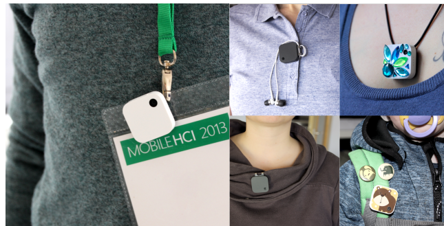
Figure 1: Camouflage of lifelogging cameras: unobtrusively attached to an event badge, paired with headphones to be mistaken as audio player, disguised as jewellery, worn on same-color clothing and decorated with stickers and hidden amongst buttons and pins. [left to right, top to bottom]
