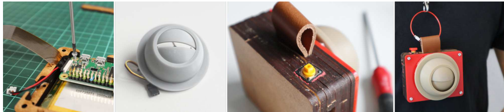
Portfolio Figure 8: To create fully functional hardware prototypes, we made use of small single-board computers (here: Raspberry Pi Zero) that enable basic image processing routines in real time. This allowed the camera to be face-responsive (c.f., Darrell et al. [DTB + 02]), and react, e.g., by closing the camera’s “eye”, to bystander presence or conversations [MSK + 18]. Cases were constructed from plywood, acrylic glass, and 3D printed parts, which creates a mixed fidelity, and “prototypical” look-and-feel.
