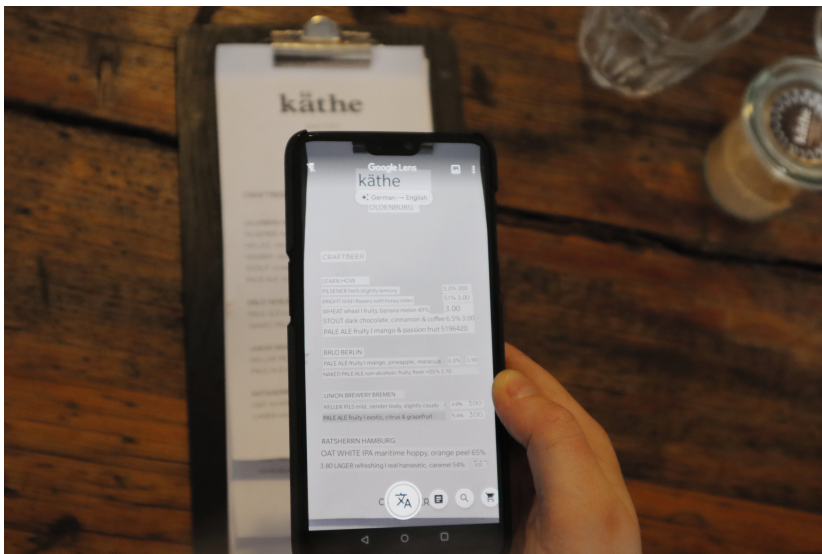
(b) The menu's text is detected from the camera's image. Its translation is then superimposed on the original frame. Image taken 2019 at Käthe Kaffee Oldenburg, Germany.
